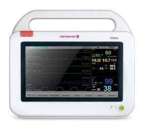
The **Omni™** offers a 3, 5, and 12 lead ECG platform. Arrhythmia detection and ST are also standard and measurable on all lead sets.
